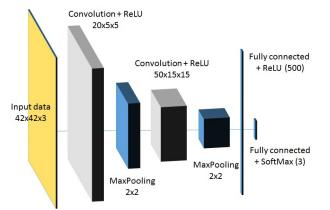
Fig. 8: Layer configuration of the LeNet CNN applied.
