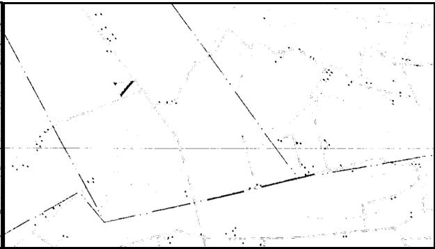
(b) Erosion operator to remove most road pixels
