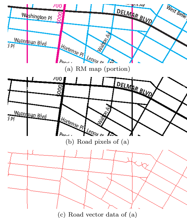
Fig. 33 Examples of the road vectorization results on the RM map
