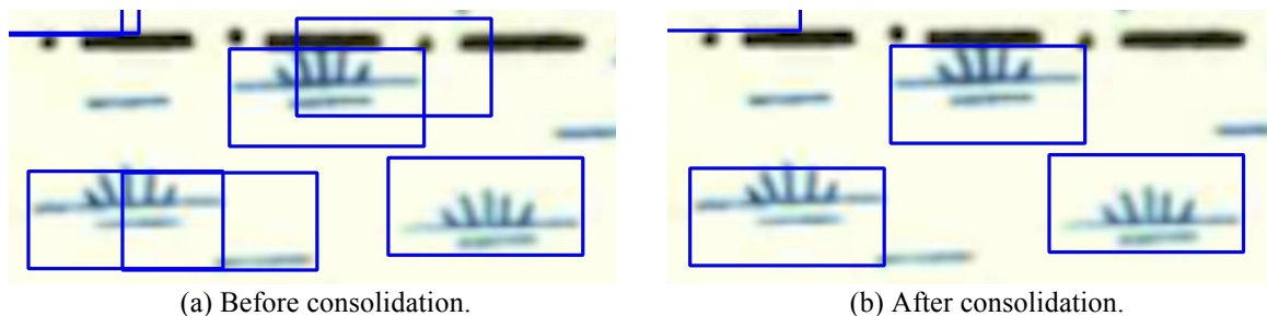
Figure 7: Result consolidation for overlapping sub-images.
