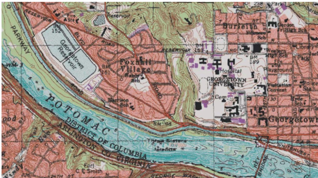
Figure 21 An example of USGS DRG based on a color scheme of 13 known colors to represent map layers 8
