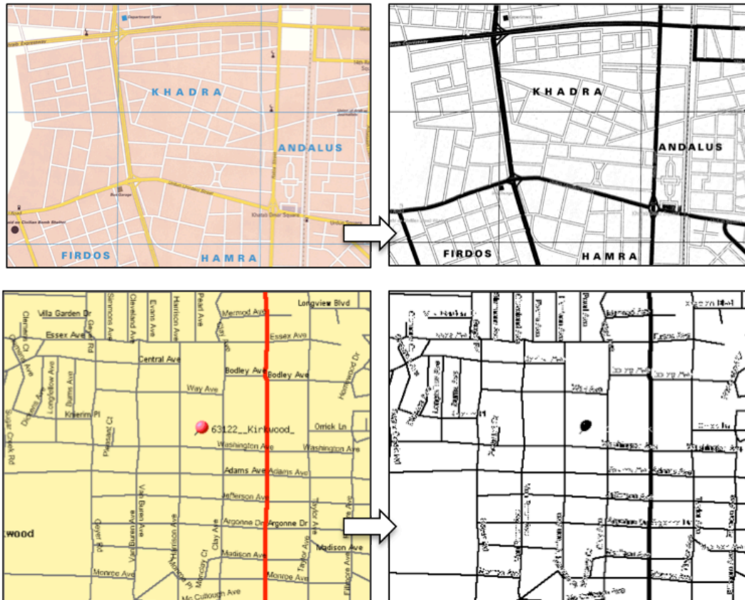
Figure 20 Sample maps and their road layer extracted with manual grayscale histogram thresholding
