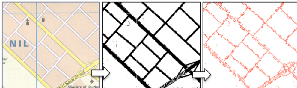
Figure 23 A sample map processed by the automatic vectorization function in R2V
