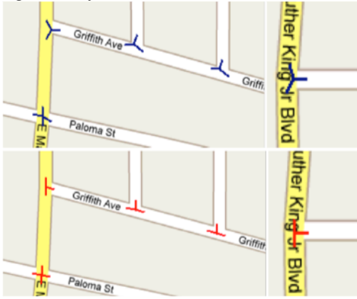
Figure 22 Automatic repairing the road geometry (Chiang and Knoblock, 2008)
